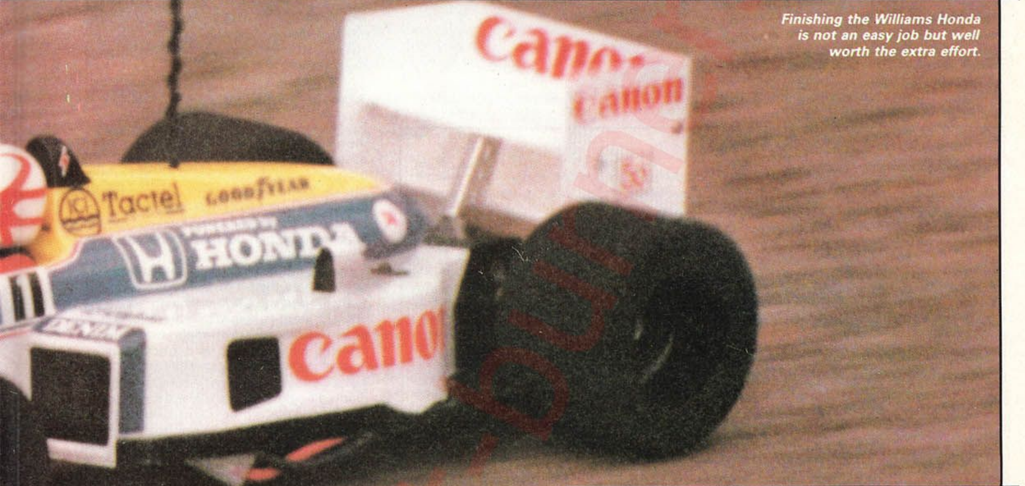
The lexan guard prevents small pieces of grit and stones from entering the exposed differential and adds to the scale appearance.
